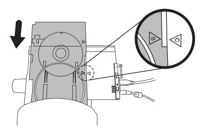
7. Click the "Tray Out" button so that the tray is pulled into the Autoloader
